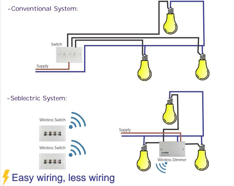
All lighting is simply wired to a Seblectric dimmer. Switches are placed wherever you want and require no wiring at all. This gives total flexibility as each switch can even be reprogrammed at a later date if you would like to alter the function of a switch. You are saving the wiring from all the switches to your lighting!
